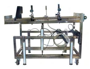
**Remote Firing Stand** shown with the protective cover removed for illustration purposes only.
